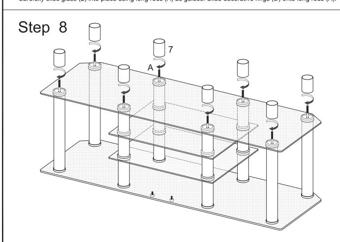
Screw cylinders (7) onto long rods (A). Cylinders (7) will fit snuggly into the decorative rings placed in the previous step.
